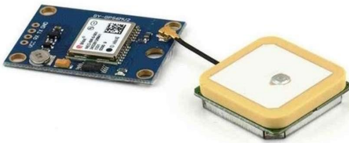
Fig. 4 GPS module with antenna
